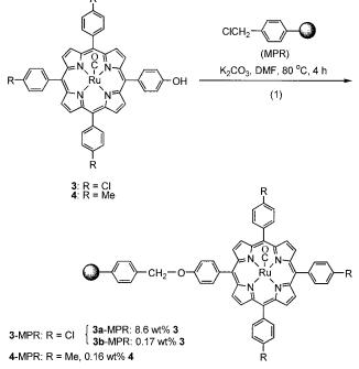
**Figure 2.** Synthesis of ruthenium porphyrins covalently immobilized onto Merrifield's peptide resin.
